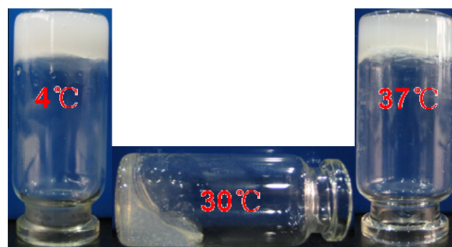
Fig. 1. The gelation process of chitosan/dibasic sodium phosphate formulation as in function with temperature from 4 to 37 °C. (For interpretation of the references to colour in this figure legend, the reader is referred to the web version of this article.)
